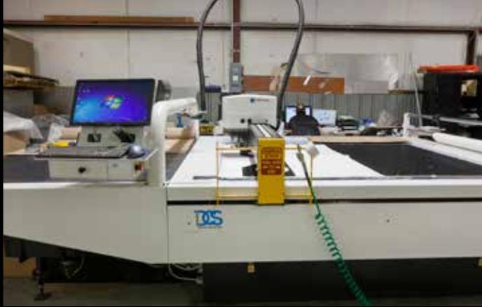
PRECISION UPHOLSTERY MANUFACTURING. THE PATHFINDER CNC CUTTING TABLE ALLOWS OUR DESIGN TEAM TO SET THE CURVE IN PONTOON DESIGNS.”
